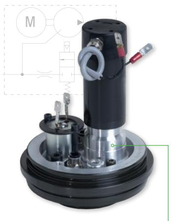
Hydraulic power pack for oceanographic buoy
