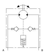
For **bi-directional** applications, the motor is fitted with an accumulator integrated in the back piece, to compensate possible pressure peaks in the housing (for example from rapid change in direction).
