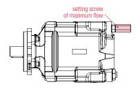
DELTA 40: can be set from 40 to 25 cc/rev DELTA 60: can be set from 60 to 35 cc/rev DELTA 75: can be set from 75 to 55 cc/rev DELTA 92: can be set from 92 to 70 cc/rev
