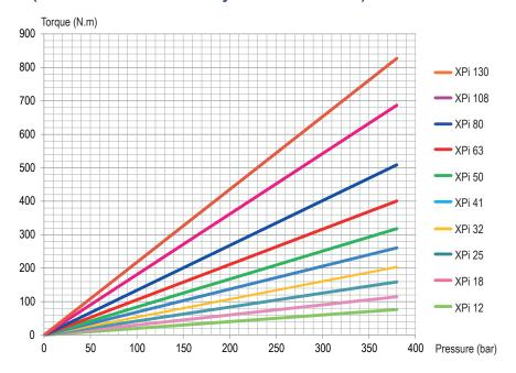
$$C = \frac{\text{Cyl x } \Delta P}{62.8 \text{ x } \eta_{\text{meca}}}$$
